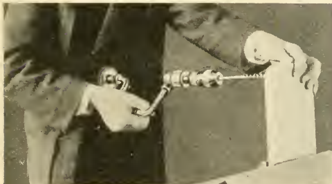
Fig. 10. Feeling for the Point of the Bit.
